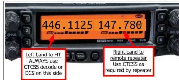
Figure 5: Mobile config for half (one way) mode
