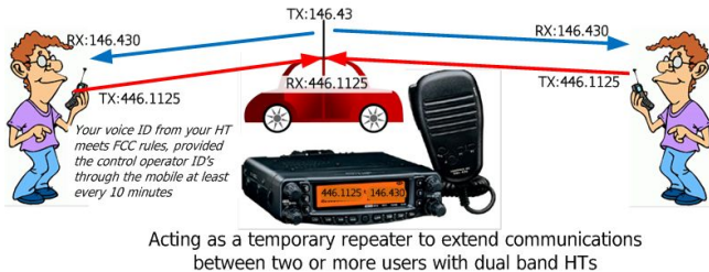
Figure 7: Temporary Repeater Mode
