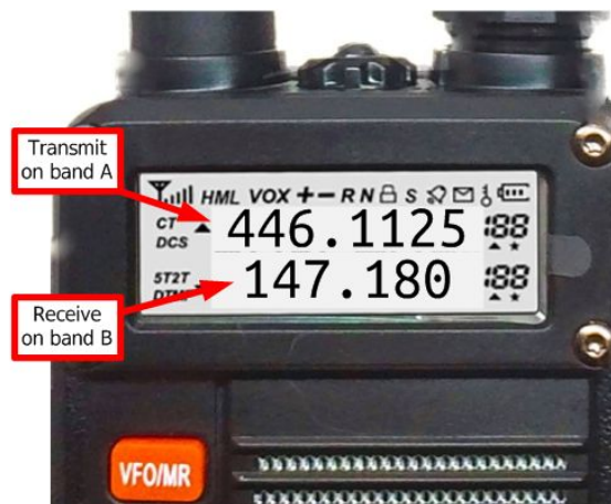
Figure 6: HT config for half (one way) mode
