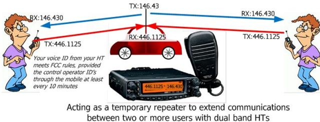
Figure 7: Temporary Repeater Mode
