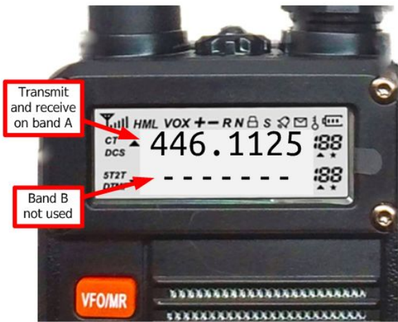
Figure 3: HT config for full (two way) mode
