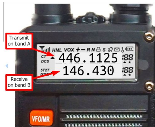
Figure 9: HT config for temporary repeater mode
