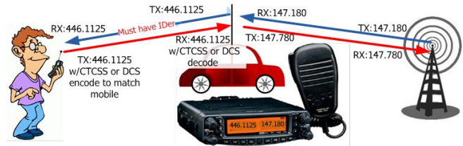
Full (two way) Crossbanding to reach a distant repeater Mobile must have built-in ID'er to meet FCC rules when using this mode
