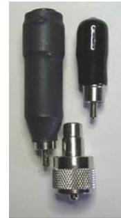
Also needed is the construction of the WA8MKH design adapter shown in a previous article and above. This is about a one foot long RG58 coax with 3 inch leads. Optional, the MFJ Model 66 Dip Adapter is shown on the far right.
