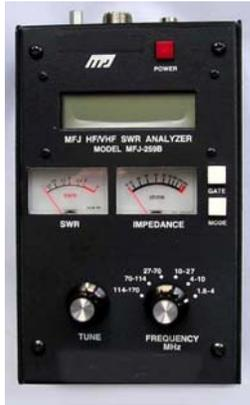
The MFJ Model 259B Analyzer is the measuring instrument used with the following construction projects. The MFJ Models 259 or 269 or similar analyzer may be used.
