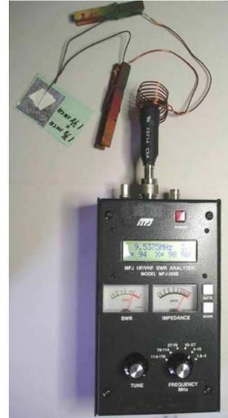
Testing resonant frequency using the WA8MKH adapter on left and top. The MFJ Model 66 Dip Adapter on the right works best slightly inside of a coil. Start with the lowest frequency on the analyzer. Rotate TUNE slowly higher in frequency until a dip in the SWR meter is noticed. Note:
