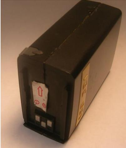
A little effort with a large bladed screwdriver enabled me to break open the case. Remember, Engineering rule No 17 states you have to **BREAK THINGS OPEN** to find out how they are made before you can fix them. I found 6 AA Ni Cad batteries with welded solder tabs, soldered up in series making the 7.2 volt battery pack.
