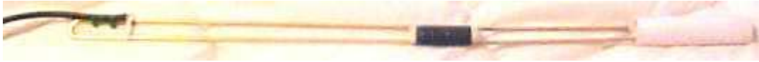
Above: Hairpin rod assembly with cable, spacer and top pvc/threaded screw assembly
