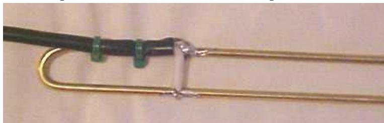
After the epoxy has completely set, measure 1 1/2 inches from the bottom of the rod (where the “U” bend is) and solder a 4 foot length of either RG-8X or RG-58 cable with the shield soldered to the SHORTEST length of rod and the center conductor soldered to the longest run (the run with the brass screw assembly). See above pix
