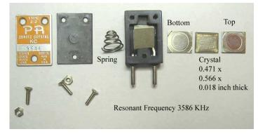
which are inserted between the 2 metal plates within the holder. The spring puts the correct amount of pressure between the cover and the crystal. An interesting note is that the crystal shown has some pencil lead marks, a techniq ue used to lower the frequency a few KHz. Special grinding would raise the frequency y.
