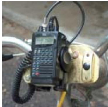
Ah, the "heart" of it all the two meter rig mounted on the front "console"
