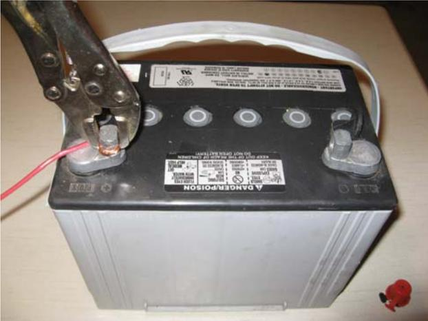
A more permanent attachment method uses Car Battery clamps and a 5 way binding post. See figure 2. Neither method works well if the battery is still connected to an automobile.
